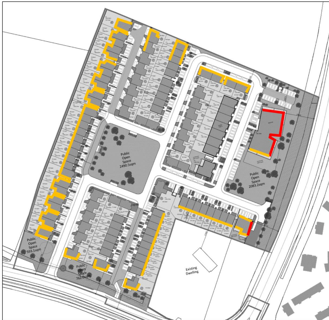
Figure 12.8: Facades Requiring Enhanced Acoustic Façade Specification (north site).
